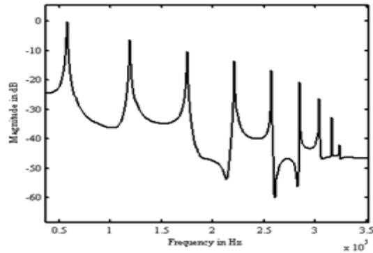
Fig.10 Winding current of DUT 2 in frequency domain with LI excitation
