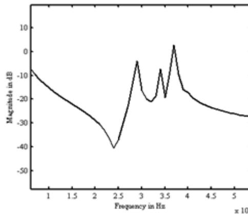
Fig.8 Response of DUT 1 with OLI excitation
