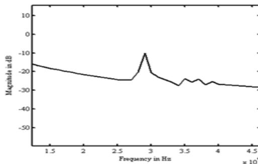
Fig.7 Winding current of DUT 1 in frequency domain with LI excitation
