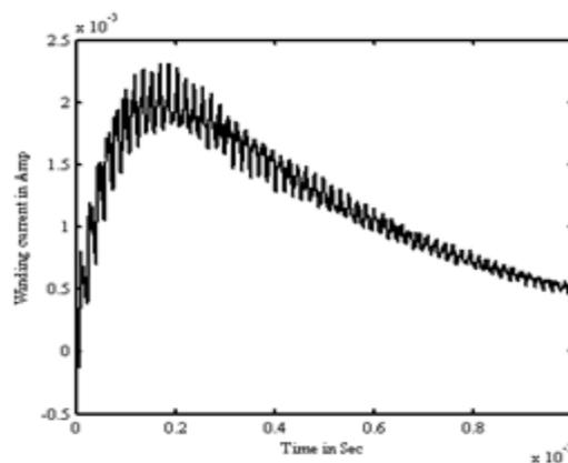
Fig.9 Winding current of DUT 2 in time domain with LI excitation
