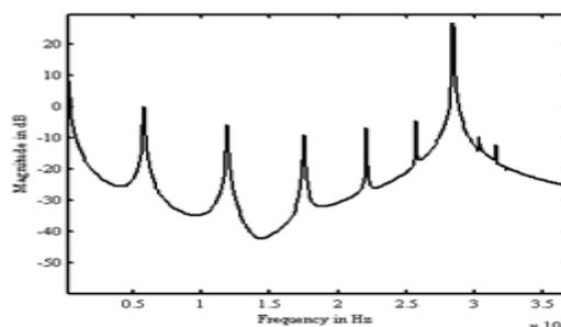
Fig.11 Winding current of DUT 2 in frequency domain with OLI excitation
