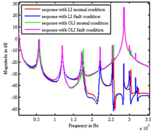
Fig.12 Response of DUT 2 for LI and OLI excitation under no fault and fault condition
